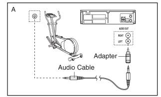
B. Plug one end of the audio cable into the jack beneath the console. Plug the other end of the audio cable into the adapter. Plug the adapter into an RCA Y-adaptor (available at electronics stores). Next, remove the wire that is currently plugged into the AUDIO OUT jack on your VCR and plug the wire into the unused side of the Y-adaptor. Plug the Y-adaptor into the AUDIO OUT jack on your VCR.
